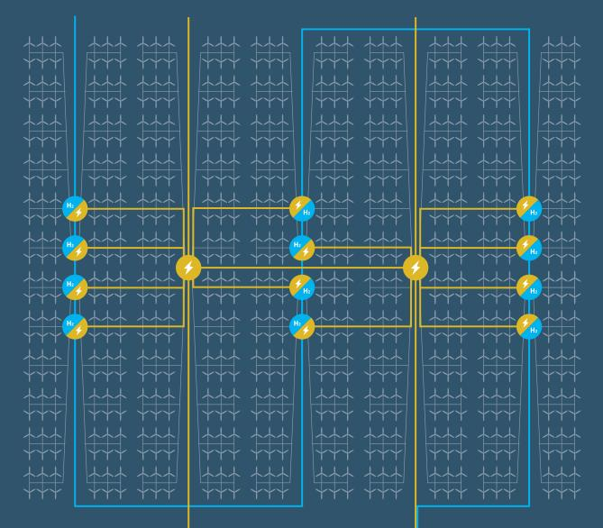
Example of large modular hub with several power and hydrogen converter stations
