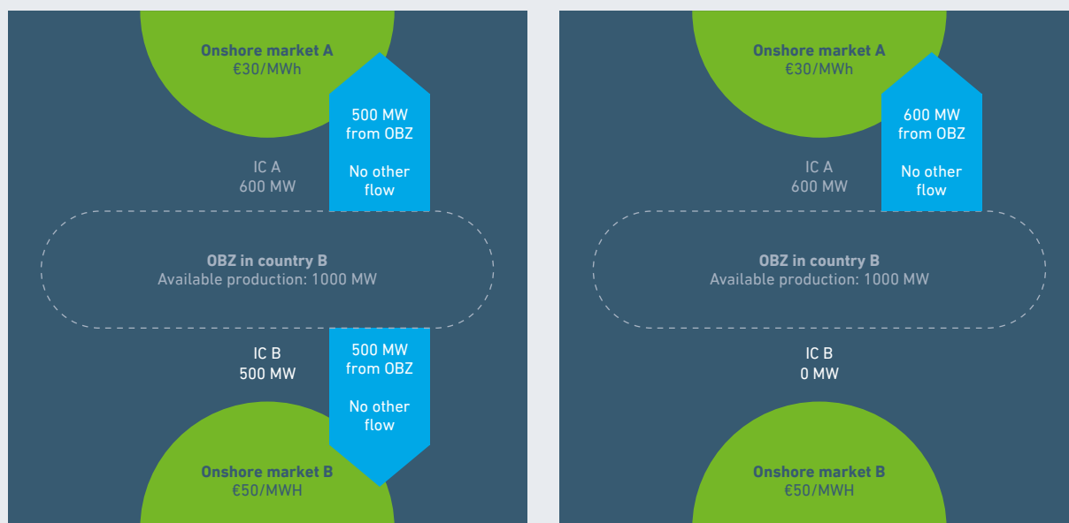
Figure 9: Worked example B: jointly sufficient export capacity.
