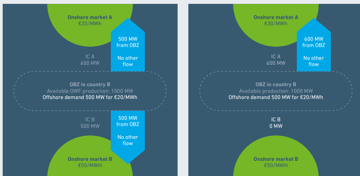
Figure 10: Worked example C: jointly sufficient export capacity including demand in the OBZ.
