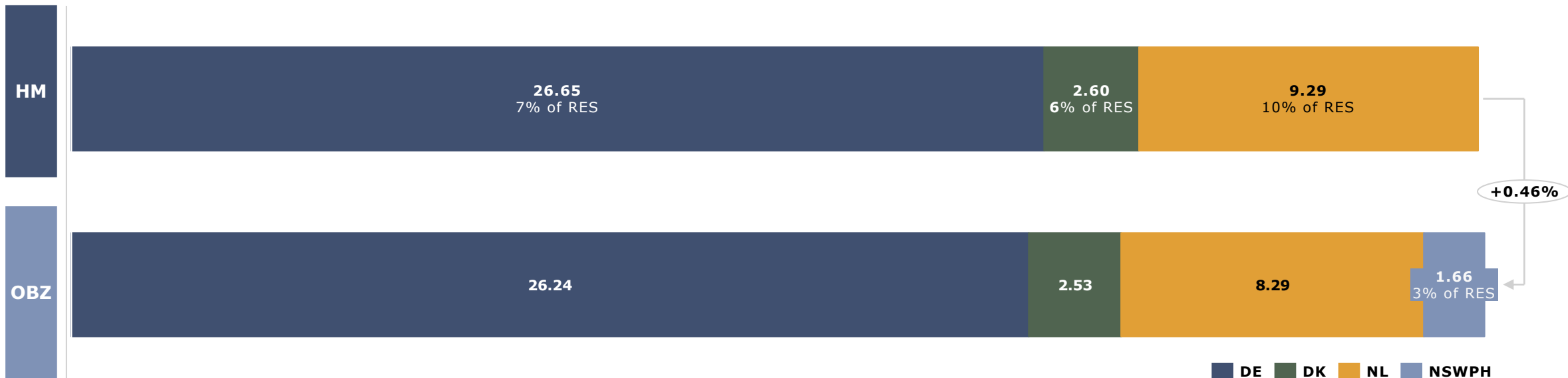
Overall RES (total wind & solar PV) curtailment levels for the core markets and the NSWPH in TWh
